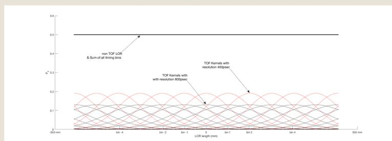
The sum over all TOF bins should be the non-TOF LOR, as demonstrated in the figure above, for two timing resolutions 600 psec and 400 psec.
