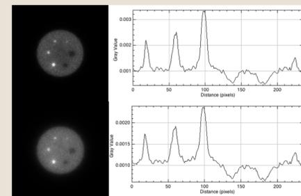
The Figure on the side present MLEM reconstructed images with and without TOF, after 8 iterations. For the hot source with radius 5mm the CRC is about 0.77 with TOF and 0.4 without. The SNR values are
