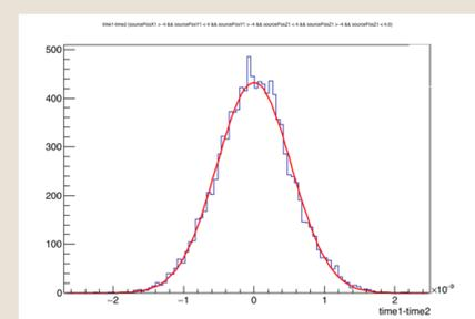
DeltaT for events originates from near the center of the FOV. Fitting demonstrates  $\sigma = 580\text{ps}$
